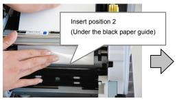
5. Remove a paper fixed tape, and insert the paper.
