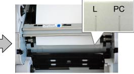
6.Fit the paper to the proper position for each size. L size and 2L size correspond to the line of L, and PC size and A5 size correspond to the line of PC.
