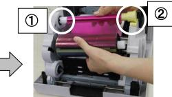
8. Set the take-up side core of the ribbon to the printer. Insert the protrusion of the core left side in the hole on the printer, then set the right side to the holder of the same color (yellow).
