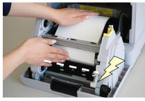
Insert the paper under the black paper guide until the buzzer beeps (approx. to the dotted line). Make sure to insert the paper straight.
